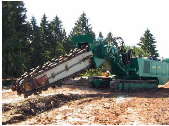
图 12-30 Trench Mechanic 止水帷幕切削搅拌设备
